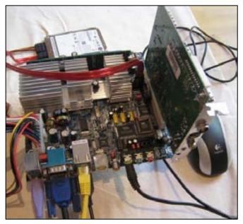
one, but you might have SATA or IDE. There is a spare Molex power connector on the ATX loom to provide power to the drive, though you may need an adapter cable for SATA. There's a second SATA plug next to the one you've used for the hard disk, or use one of the blue IDE connectors on the edge of the board near the memory slot.
