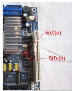
f. Pull the jumper back off the pins, and re-insert it – this time on the two pins further from the battery holder, where it probably started.
