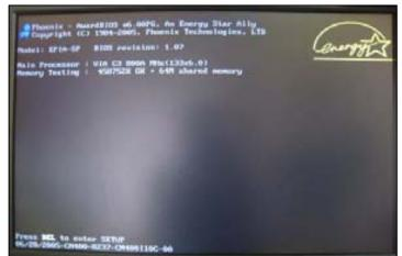
starts you can set the screwdriver down. When successful, there is a quiet 'click' sound and the motherboard will start up. When the boot screen (right) is displayed on your monitor, press 'Del' or 'Delete' immediately.
