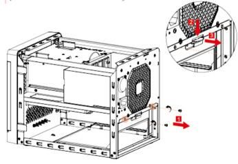
Release one screw and remove the expansion card cover.
