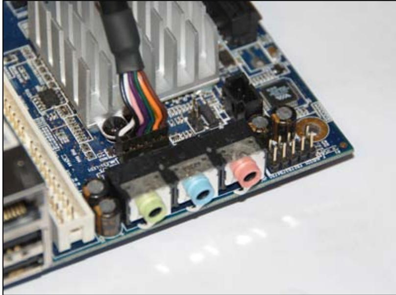
3. Connect the other end of the cable to EPIA SN motherboard as shown in the diagram above.
