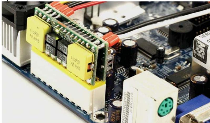
2) Connect a 12-25VDC power adapter (peak should not exceed 26.5V) to the input connector.
